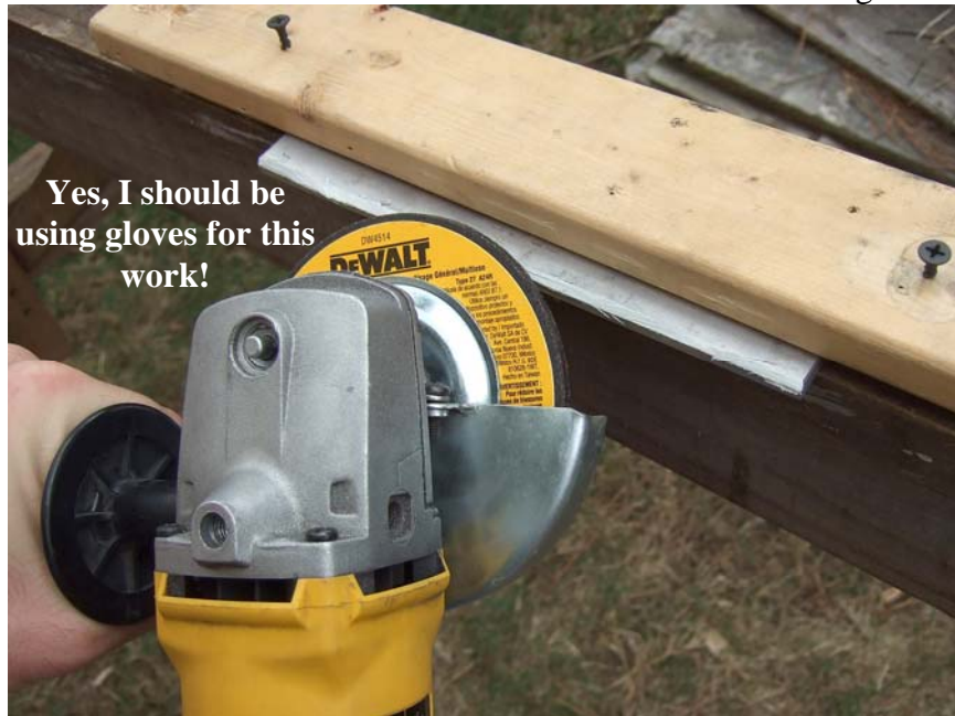
Using angle grinder instead of the bench grinder
