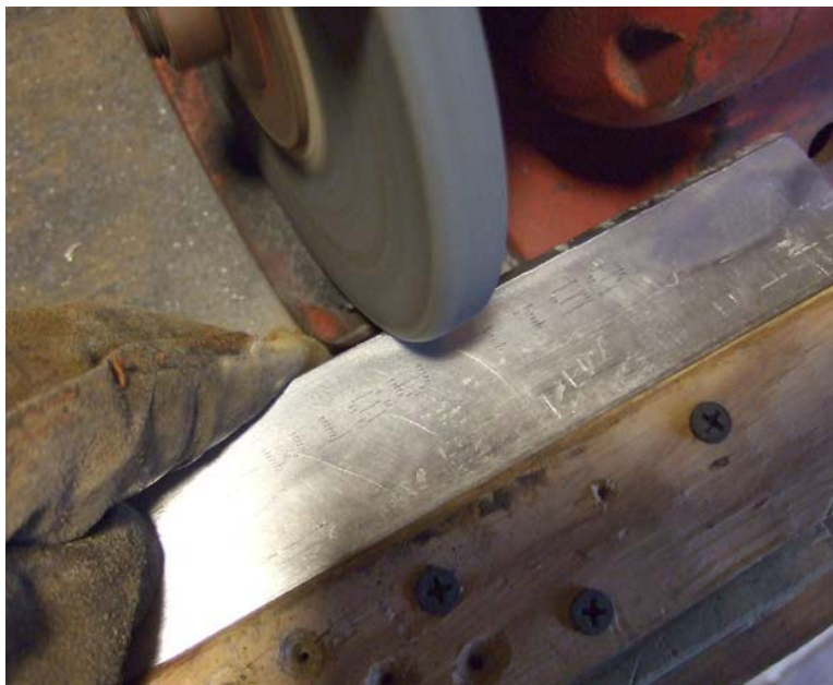
Beveling the edges with the grinder
