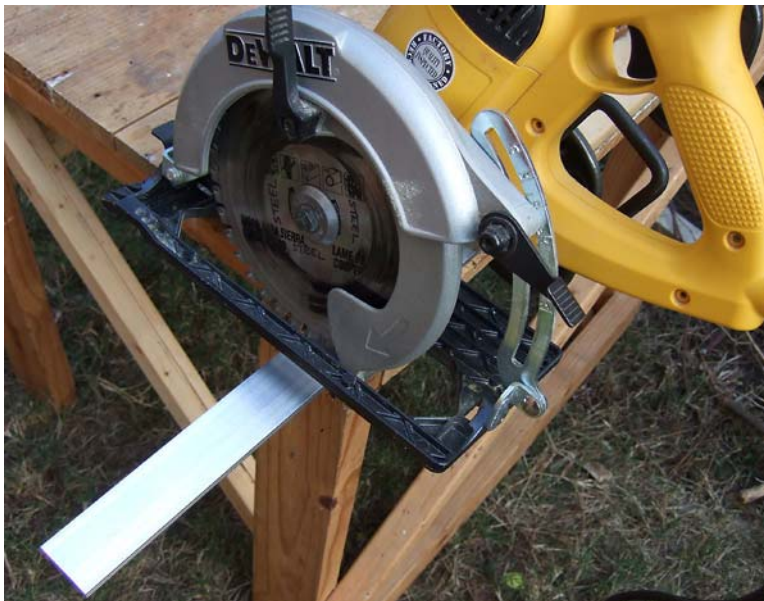
Cutting approx. 8-inch long work piece from flatbar stock
