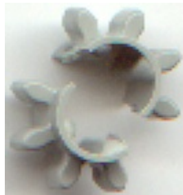
Broken 8t gear
